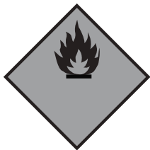
FLAMMABLE LIQUID FLAMMABLE GAS FLAMMABLE AEROSOL
